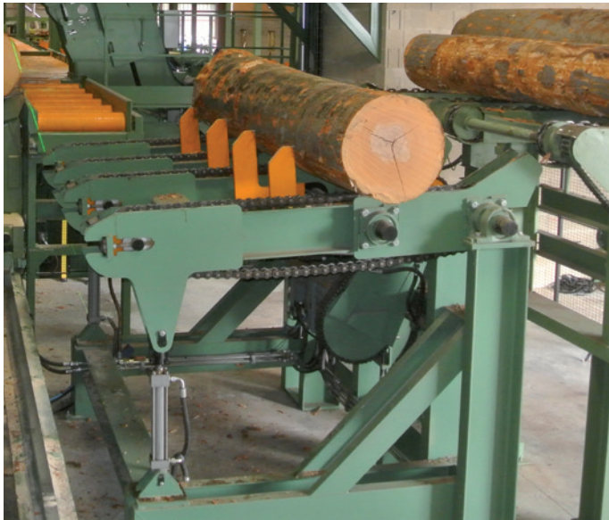
Motorized Loading system for Hardwood equipped with flighted chain and stoppers.
