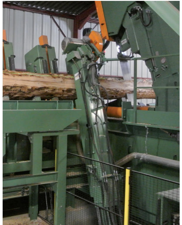
Installed before the headrig for pre-edging and cutting slabs and other products, thickness up to 150 mm.
